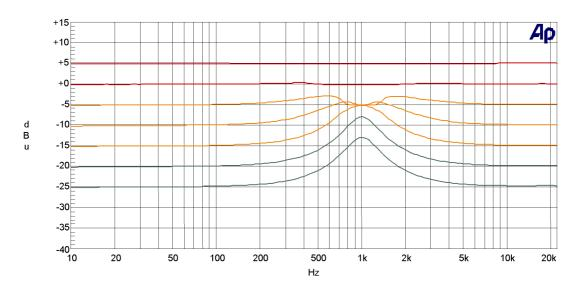
In this example, [low threshold] is -20dBu, [low level] is +12dB, [high threshold] is set to -5dBu, and [high level] is 0dB. Thus, the lowest trace shows an input at -25dBu with a standard parametric boost of +12dB at 1kHz. The -20dBu trace shows an identical response, as expected. However, once above this level the filter gradually fades out with increasing signal, until at all levels above 0dBu the response is flat.
